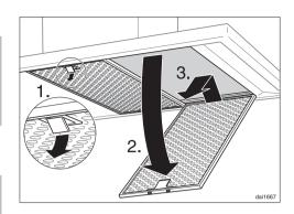
■ To take out the grease filters, release the locking clip on the filter, lower the filter 45°, unhook it at the back and remove it.
